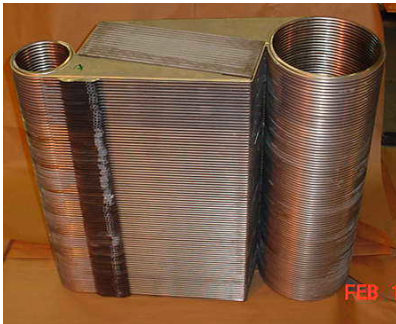
Ingersoll-Rand Recuperator core
